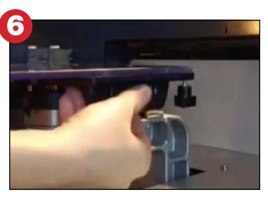
Secure the Platen Insert by rotating the center piece in the T-Lock brackets.
